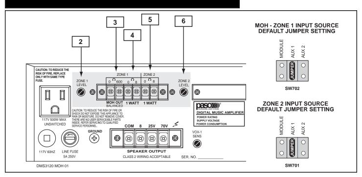
Fig. 24 - Rear Panel View - ZONE 1 - ZONE 2 - MOH Outputs - Source Selectors and Controls
